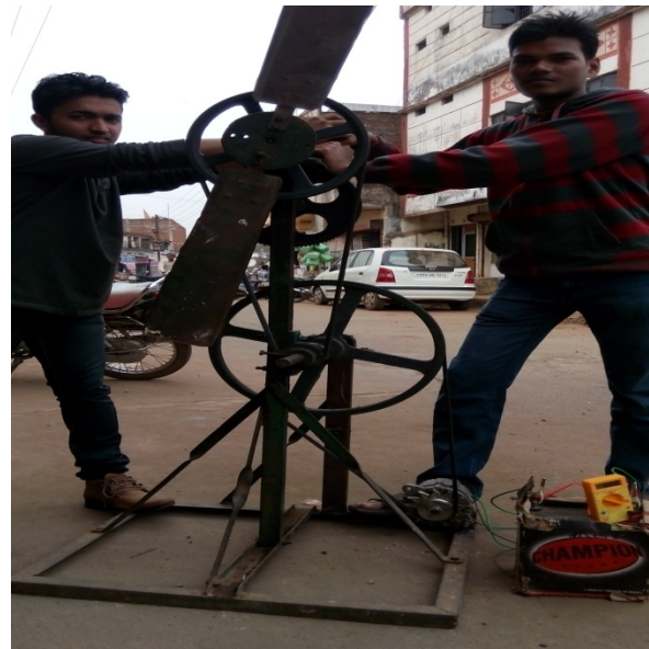
Fig. 2 : Human powered winnowing fan for generating power.
