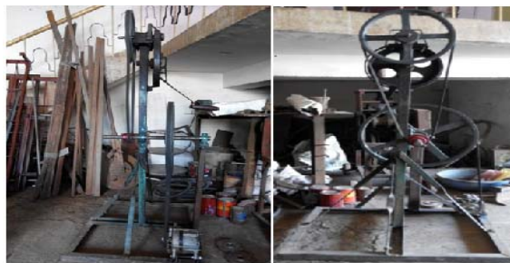
Fig. 1: Side and Front view of hand wincrowing fan.
